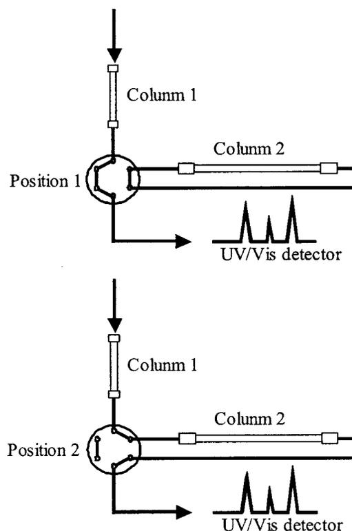
Figure 2. Schematic diagram of the HPLC system used for the determination of anthocyanins in plasma and urine from humans and rabbits.
